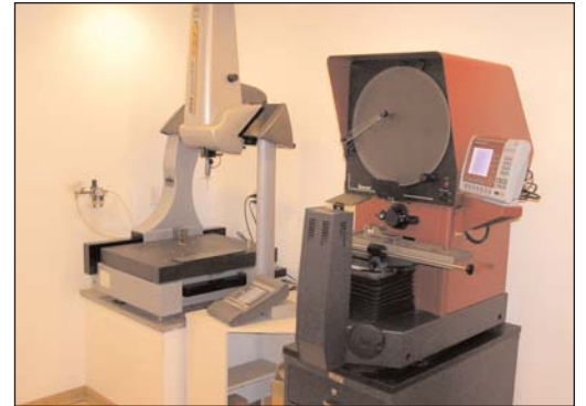
Optical Comparator and Coordinate Measuring machine are used for precision quality control at JT Precision, Inc.
