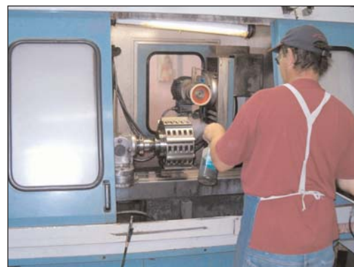
Filegar Cutting Technologies' Pat Bunce services industrial flooring head.
