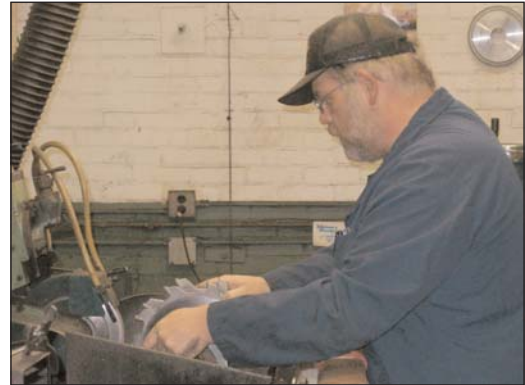
Chuck Yaw, Filegar Cutting Technologies technician, grinds profile tooling.
