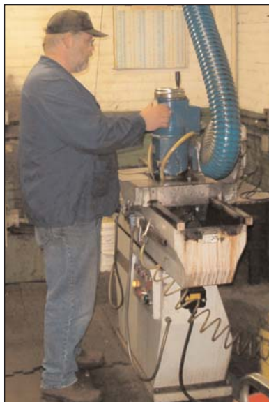
Chuck Yaw sharpens high speed steel knives.
