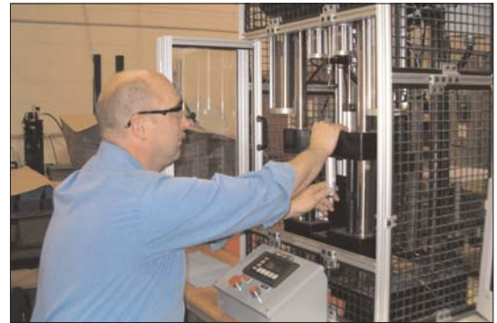
Enivate Quality Technician, Dave Bargy, tests a dashpot on a time to stroke tester.
