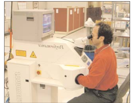
Chris Talebkah, a Sr Manufacturing Engineer at Conax Buffalo Technologies LLC, joins precise parts on a laser welding machine.
