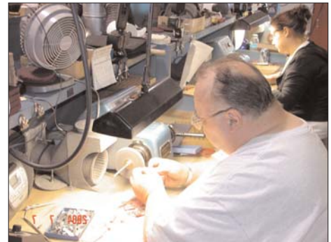
Casey Machine's Pat Obermiller (front) and Jackie Stachiewicz (back) perform deburring operation on high precision component.
