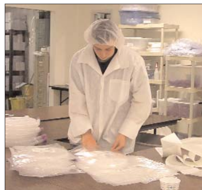
Packaging and assembly of tubing products in Buffalo Filter's Clean Environment Room (CER).
