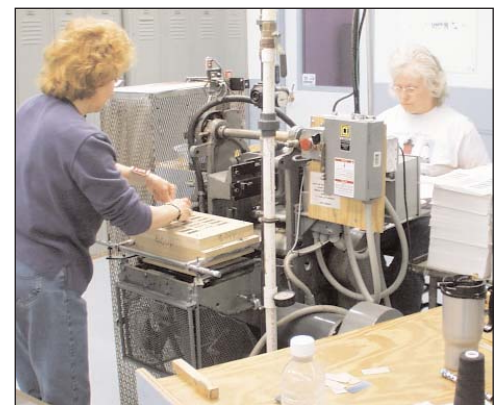
Utilizing two setup operators significantly reduced the changeover time on these machines.
