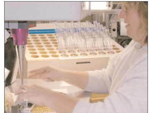
Colleen Hochadel, Polymer Conversions Technician, applies ultrasonic weld to adhere brass part to plastic housing for medical device.
