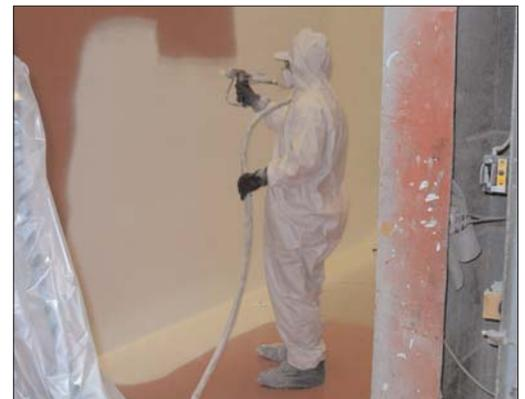
Unicell's Jose Arroyo applies gel coat to interior of truck body mold cavity prior to application of fiberglass.
