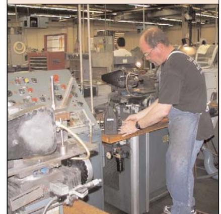
Pivot Punch technician, Bruce Smith, uses grinder to complete a punch profile.
