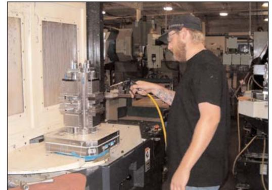
PCB Machine's Rob Muscoreil (Green Belt) prepares fixture prior to loading into horizontal mill.
