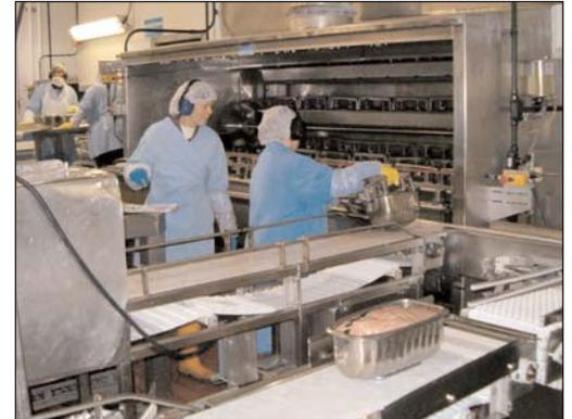
Ham mix is poured into molds prior to baking at Tyson Foods.
